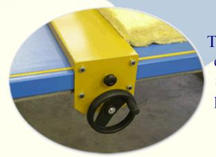
The requested size can be adjusted with an easily moveable stop block by hand. The stop block can be fixed at the adjusted position.
